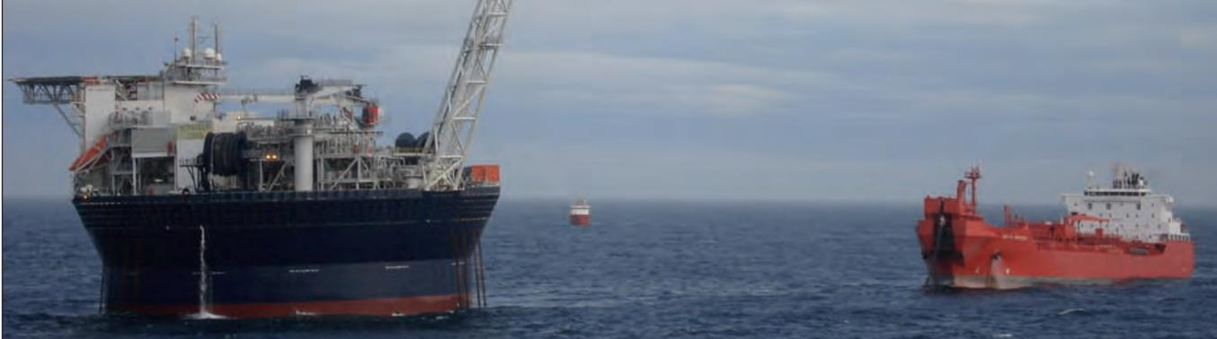
**S**evan brought the first round FPSOs into operation. While the Norwegian company may not have been the first to have thought of the round FPSO concept, it was the first to successfully develop and commercialize it. That's a remarkable achievement, for it is tough to get a novel production facility concept accepted because it requires an oil company to dedicate a field to the new technology. Success for both parties hinges on much.
