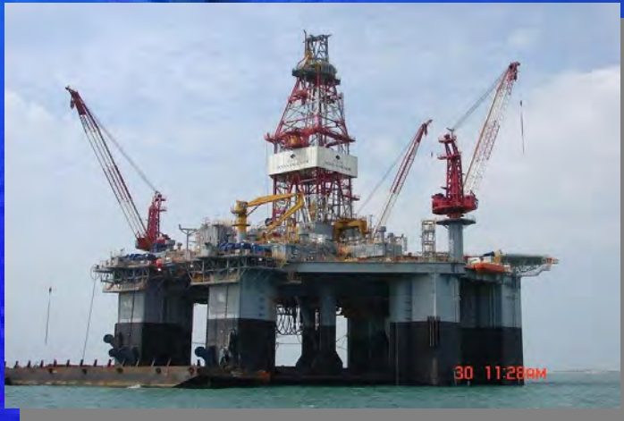
Ocean Endeavor - 10,000 ft WD ( Under Contract to Devon Energy ) Diamond Offshore Drilling
