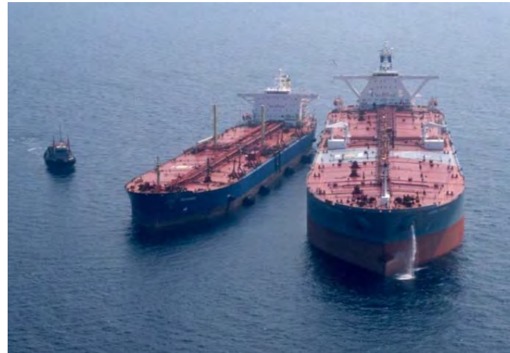
Lightering: side by side offloading VLCC to shuttle tanker size, offshore
