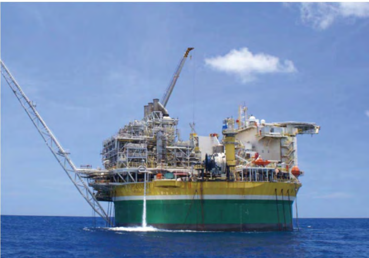
Illustration 3: First Operational Round hull for FPSOs & MODUs of Sevan Design, at Piranema Field Offshore Brazil in 2007
